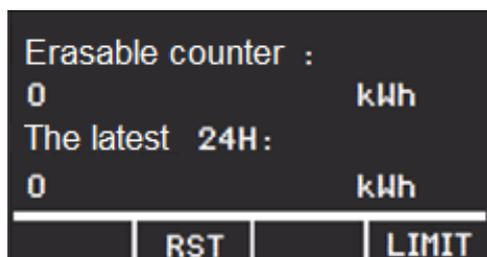
In the Boiler Working Count window, the LIMIT option is visible (bottom right-hand corner of the window). The LIMIT window is activated by pressing the Up arrow.
