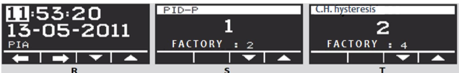
**1.3 Settings/Date and time** - on the start screen (C), press to enter into SETTINGS (J), select Date and time (K) and press again. Use ←→ (R) to toggle between time, date and day of the week, and ↑↓ to change parameter values, which are saved by pressing . Setting Auto to 1 causes the time to update automatically. This applies to boilers connected to the Internet.
