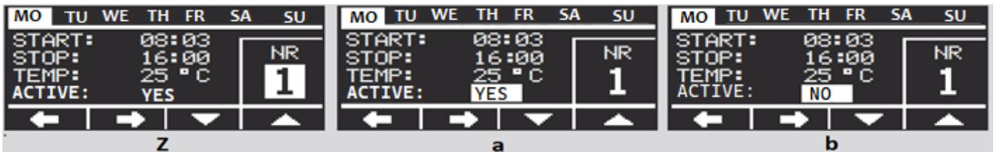
**1.8. Settings/Programmes CSP** - on the start screen (C), press the by going into SETTINGS (J), selecting CSP Programmes (L) and once again pressing the . By using  $\leftrightarrow$  (Z) toggle between the parameters (days of the week, operating hours, temperature, activity), and with the  $\uparrow\downarrow$  change the parameter values, which are saved by pressing the .
