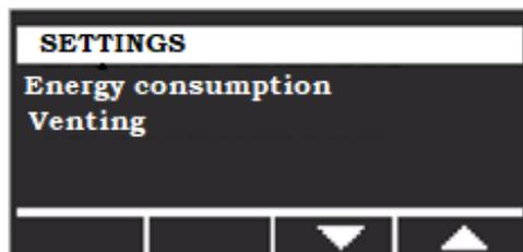
Once the above is done, you go to the Main Menu. Using the down arrow, navigate to the option: Energy consumption and press
