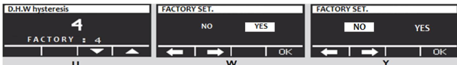
**1.6 Settings/Hysteresis D.H.W.** - on the start screen (C) press  enter into SETTINGS (J), select D.H.W. hysteresis. (L) and once again press . By using ↑↓ (U) change the value of the parameter (range 1-2-3-4-5-6, 6 is recommended), which is saved by pressing .
