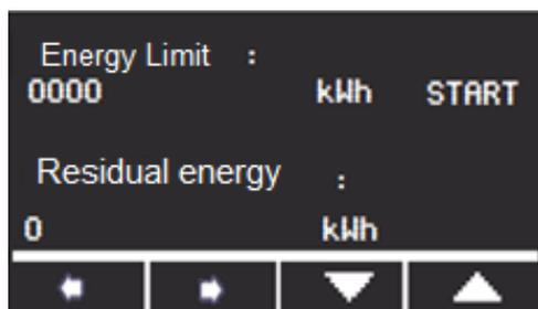
In the limit window, we set the energy value between 0 and 9999 kWh. Use the Left and Right arrows to navigate between the visible digits, while the Up and Down arrows change the value.
