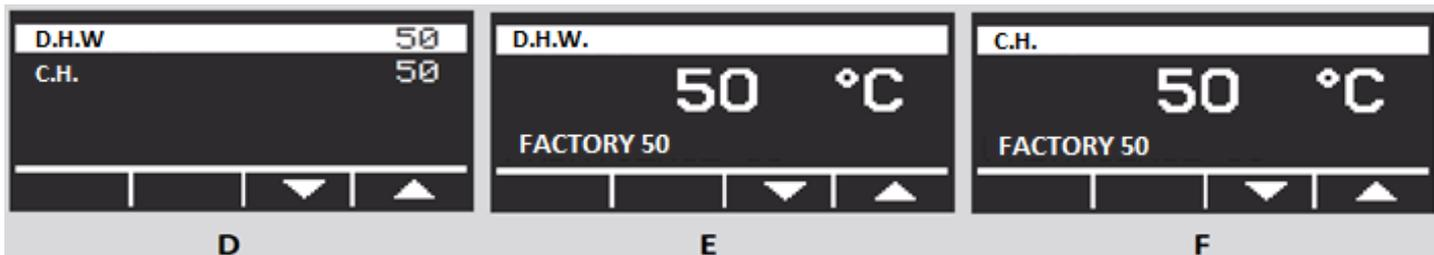
Temperature setting for **C.H.** and **D.H.W.** (for Marshal AsDC-W and D.H.W. package) - the function is accessed from the start screen (C) by pressing the ←, by using ↑↓ select the temperature for C.H. and D.H.W. (D). By pressing  enter the settings for the selected temperature (E)(F), then by using ↑↓ increase or decrease the parameter value. Temperatures are saved by pressing .
